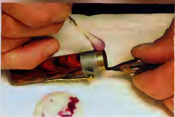
Plating supplies from left: Simichrome polish; Micromesh polishing pads; stainless steel and nickel plating solutions; gold plating solution; rotary polishing tool. Polishing the PFM clip with rotary polishing tool. Applying pre-plate solution to the PFM clip. Note negative wand attached to pen clip. Applying gold plate solution to the Ripple cap band.
